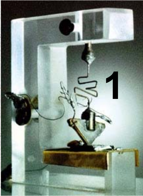
The world's first transistor (Bell Lab, 1948-50), Nobel Physics Prize 1956
