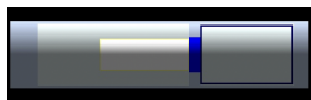
Figure 2: Side view of the N16 source geometry. The decay chamber is shown as the rectangle on the right while the small rectangle on the left represents the PMT. [2]
