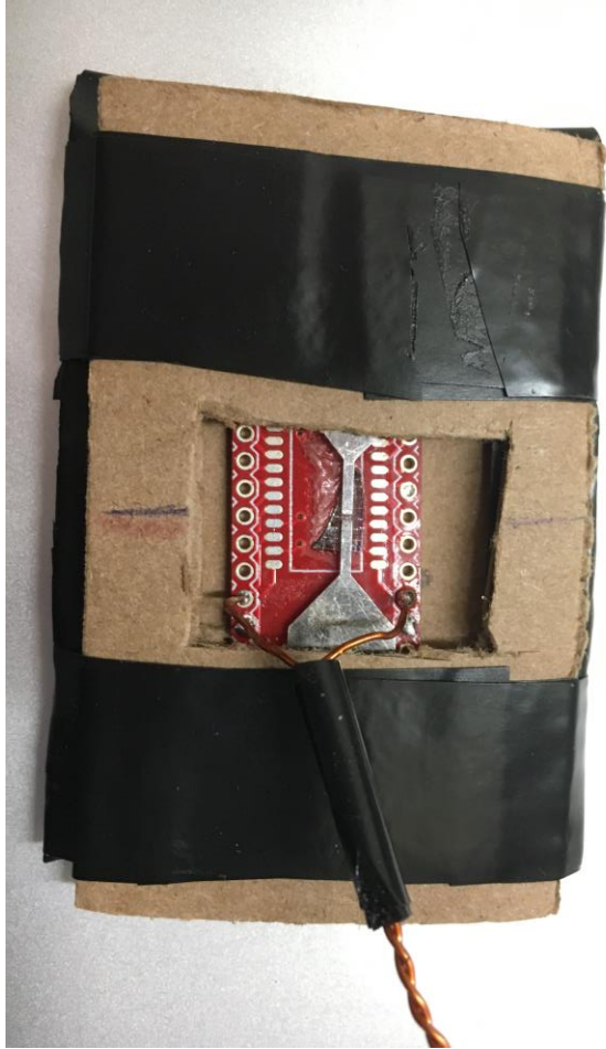
The MTJ sensor with 2 nd concentrator
