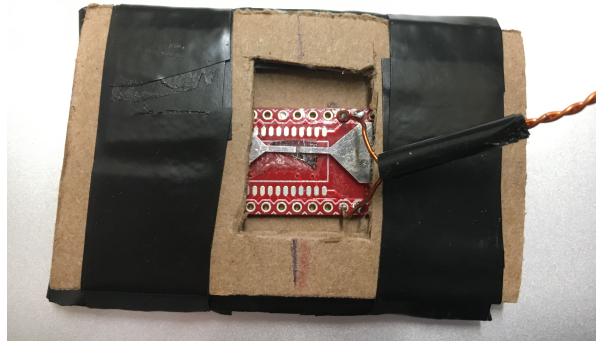
FIG. 5. The MTJs sensor with two secondary concentrators.
