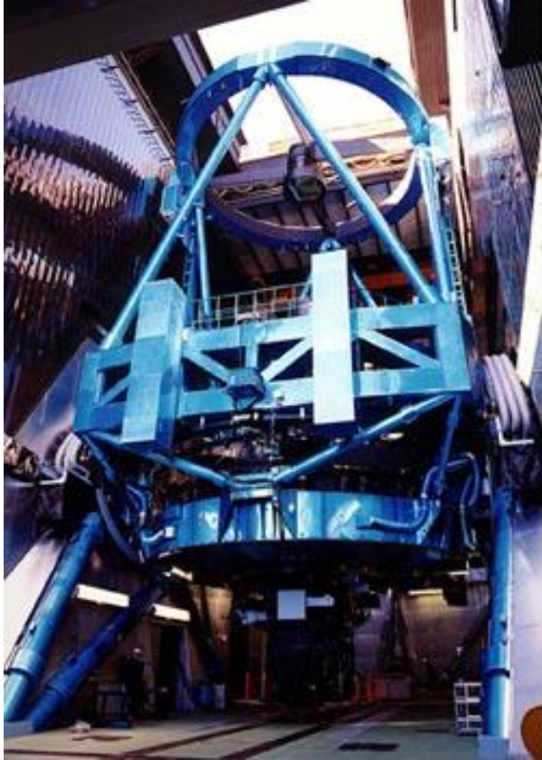
Subaru Telescope Effective diameter: 8.2 m Focal length: 15 m
